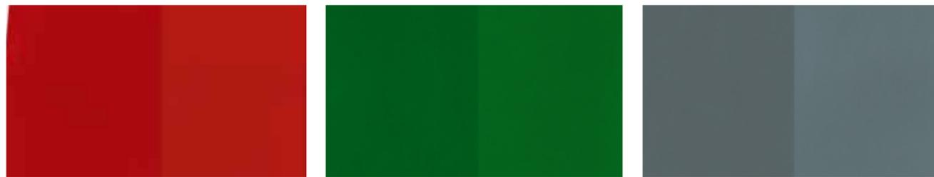
Color development of pigment preparations (left) vs. pigment blends (right). The pre-dispersed dry preparations develop the full colour strength even by applying low shear forces.
